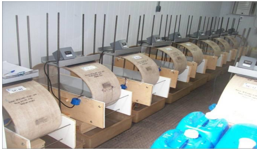
Strain-corrosion testing per ASTM D 3681, showing the deflected pipes exposed to 5% solution sulfuric acid.
